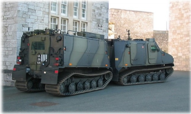
BV206 Haggglunds over snow vehicle, which is mainly used in Norway to tow the 105 Light Gun. It is also described/known as a Gun Limber or simply a gun-towing vehicle
