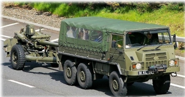
The regiment uses the Pinzgauer 716M model as a gun-towing vehicle for all other terrains
